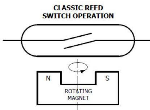
As reed switches are mechanical devices, they have a finite lifespan, with fatigue and breakage likely after around  $10^9$  operations under ideal conditions. The contacts should be protected by a current-limiting component to prevent a voltage supply being directly switched, causing them to weld together. In hazardous atmospheres, this extra protection may prevent an intrinsically safe instrument from reading the contact closures and so should be removed.
