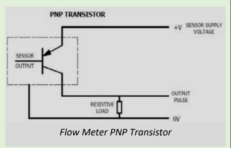
These types of sensor are used extensively in mechanical flow meters due to their reliability, clean square wave and long life. They are also able to measure very high frequencies so often found in high-rate turbine systems where you can have in excess of 1kHz pulse generation required.
