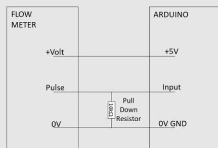
Note: For NPN the 10K Ohm resistor can be omitted if the Arduino's internal pull-up resistor is enabled
