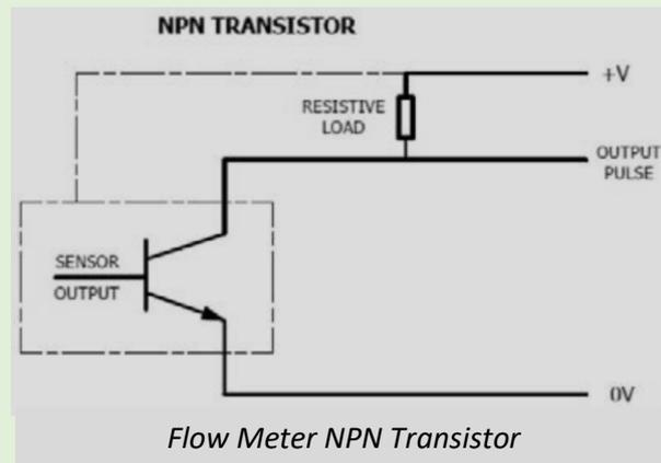
For example, using 24 volts can allow for safer transmission over longer distances. The exact value of the resistor is typically not critical, though it needs to be large enough to limit the current at the chosen voltage (within the specified limit), and small enough to provide sufficient current to activate the switch. Typical pull-up resistor values are between 1K and 50k Ohm.
