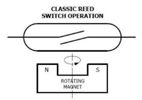
As reed switches are mechanical devices, they have a finite lifespan, with fatigue and breakage likely after around 10<sup>9</sup> operations under ideal conditions. The contacts should be protected by a current-limiting component to prevent a voltage supply being directly switched, causing them to weld together. In hazardous atmospheres, this extra protection may prevent an intrinsically safe instrument from reading the contact closures and so should be removed.
