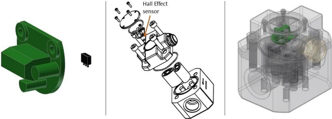
Hall Effect Sensor placement in an Oval Gear Flowmeter
