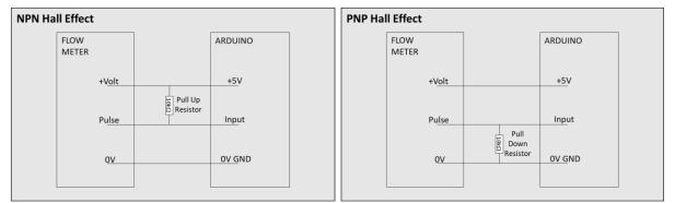
Note: For NPN the 10K Ohm resistor can be omitted if the Arduino's internal pull-up resistor is enabled
