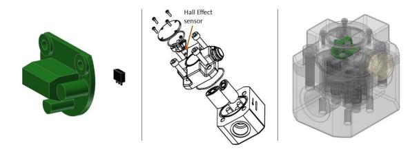
Hall Effect Sensor placement in an Oval Gear Flowmeter
