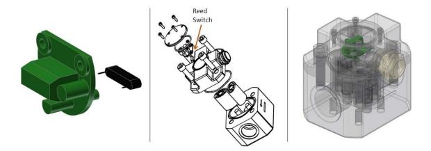
Reed Switch placement in an Oval Gear Flowmeter
