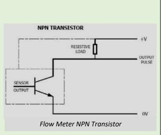
For example, using 24 volts can allow for safer transmission over longer distances. The exact value of the resistor is typically not critical, though it needs to be large enough to limit the current at the chosen voltage (within the specified limit), and small enough to provide sufficient current to activate the switch. Typical pull-up resistor values are between 1K and 50k Ohm.
