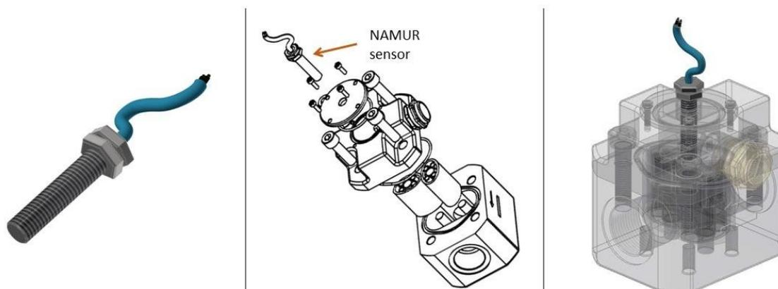
NAMUR Sensor placement in an Oval Gear Flowmeter
