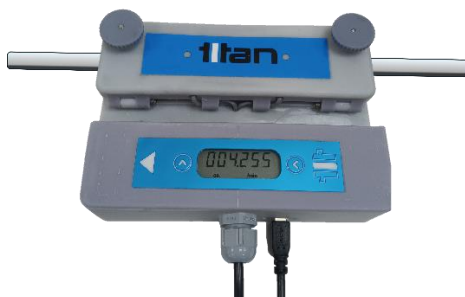
Fig 10. 3D printed clamp-on prototype with clamp sensor over silicone tube and separate display
