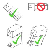
Plastic cap should always be positioned lower than flow tube and steel body
